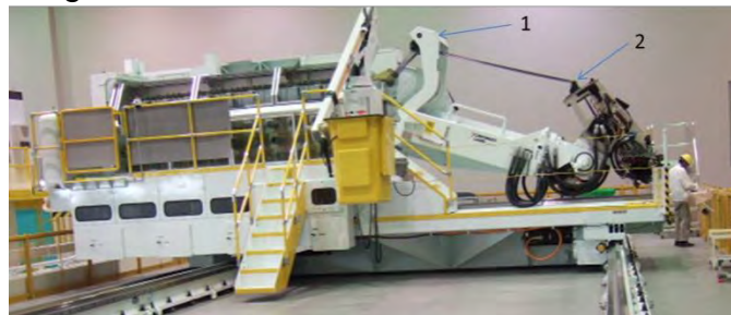
FIGURE 2 – EXAMPLE OF TYPICAL AFP MACHINE WITH MULTIPLE REDIRECTS SHOWN AT POINTS 1 AND 2 LIMITING ANGULAR MOTION
